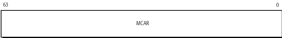
Figure 28. Machine-Check Address Register (MCAR)
