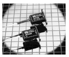
and  $625 \,\mu\text{W}$ . The "high power" LSC3100 uses the same laser chip, but with tighter fiber coupling to achieve output powers from 1 mW to  $2.5 \, \text{mW}$ .
