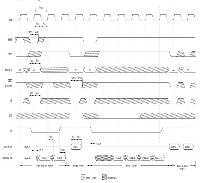
Note: 19. The data bus (Q) remains in High-Z following a Write cycle unless an ADSP, ADSC, or ADV cycle is performed. 20. GW is HIGH.
