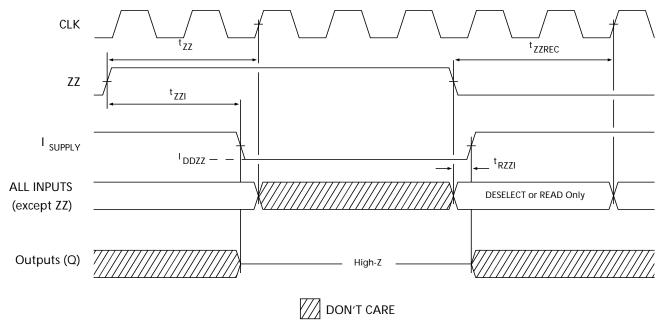
Notes: 21. Device must be deselected when entering ZZ mode. See Cycle Descriptions table for all possible signal conditions to deselect the device. 22. DQs are in High-Z when exiting ZZ sleep mode.
