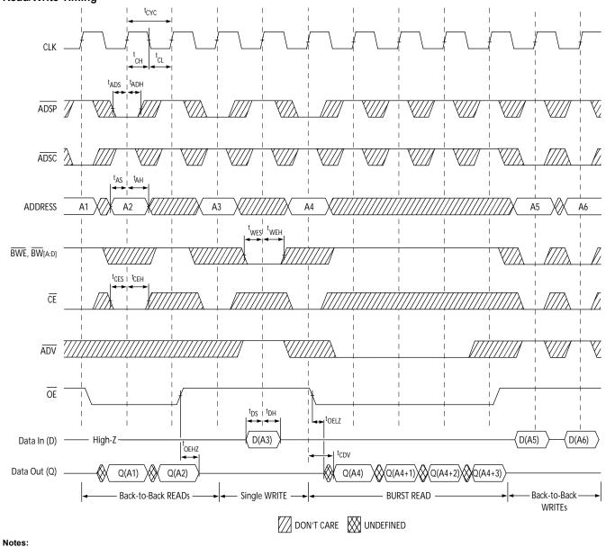
The data bus (Q) remains in High-Z following a Write cycle unless an ADSP, ADSC, or ADV cycle is performed.
