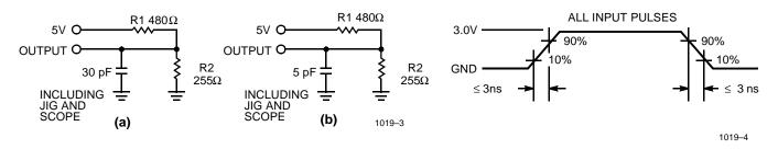
Equivalent to: THÉVENIN EQUIVALENT 167Ω -0 1.73V OUTPUT O
