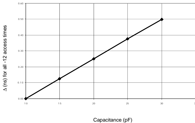
(b) Load Derating Curve
