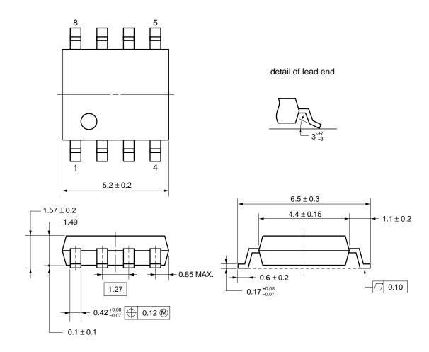
NOTE Each lead centerline is located within 0.12 mm of its true position (T.P.) at maximum material condition.
