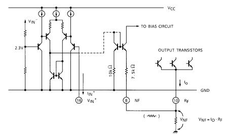
In the case of output current feedback to the motor, connect feedback resistance to  $R_{\rm F}$  pin (10) and feed it back to  $N_{\rm F}$  pin (8).
