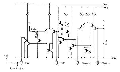
The FG amplifier is stored with internal reference voltage (2.5 V), making it possible to directly input the FG signal from pattern FG. The Schmitt circuit stored within can output wave-shaped FG signals. FGO is in push-pull mode with low impedance.
