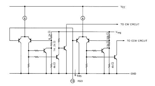
Voltage applied to FRS pin (15) makes it possible to select forward, reverse, and stop modes. For the relationships between FRS, control input, and output, refer to the item on these functions. The relationship between input voltage (V<sub>FRS</sub>) and input current (I<sub>FRS</sub>) to the DRS pin (15) is shown as a feature in the following graph:
