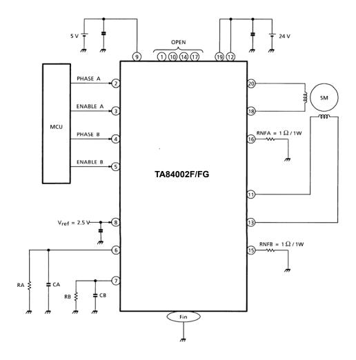
Note 1: A capacitor for noise suppression should be connected between the power supply  $(V_{CC}, V_M, V_{ref})$  and GND to stabilize operation.
