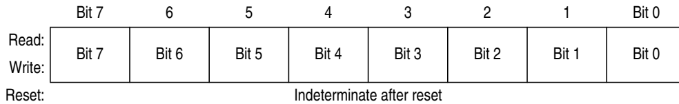
Figure 16-15. TIM1 Channel Register Low (T1CHxL)
