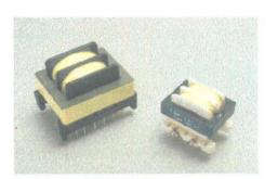
TAIPEI MULTIPOWER OFFERS STANDARD EE25.4, AND EE35 FERRITE CORE PACKAGES AND COMMON MODE CHOKES FOR USE IN INPUT FILTER CIRCUITS OF SWITCHING POWER APPLICATIONS AT 20KHZ OR HIGHER TO REDUCE AC LINE CONDUCTED INTERFERENCE.
