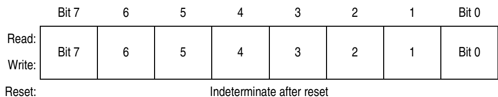
Figure 10-15. TIM Channel 1 Register Low (TCH1L)
