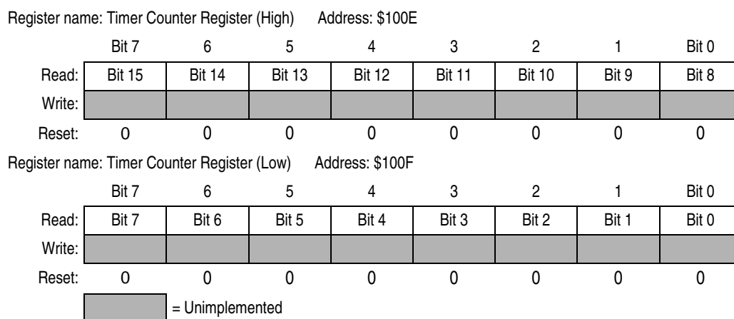
Figure 9-15. Timer Counter Register (TCNT)
