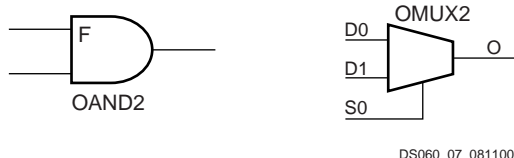
Figure 7: AND and MUX Symbols in Spartan-XL IOB
