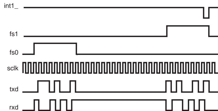
Figure 21. CODEC Interface Timing (8-Bit Mode)
