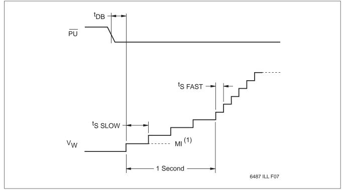
**Notes:** (1) MI in the A.C. timing diagram refers to the minimum incremental change in the wiper voltage.
