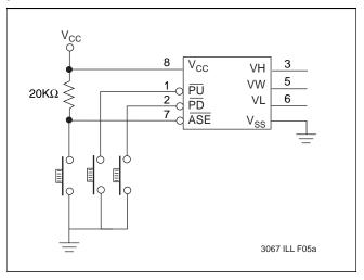
on how long the button is being pushed. When making a continuous push, after the first second, the increment/decrement speed increases. For the first second the device will be in the slow scan mode. Then if the button is held for longer than 1 second the device will go into the fast scan mode. As soon as the button is released the X9511 will return to a standby condition.
