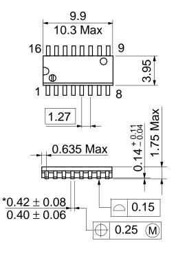
\*Dimension including the plating thickness Base material dimension
