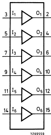
Fig.1 Functional diagram.
