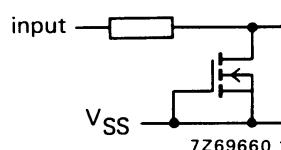
Fig.4 Input protection circuit that allows input voltages in excess of  $V_{DD}$ .**Guaranteed fan-out in common logic families**
