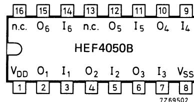
Fig.2 Pinning diagram.
