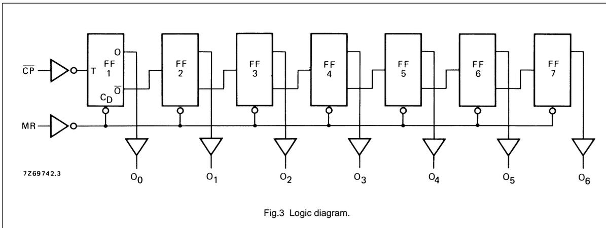
Fig.3 Logic diagram.
