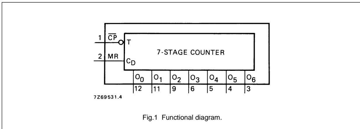
Fig.1 Functional diagram.
