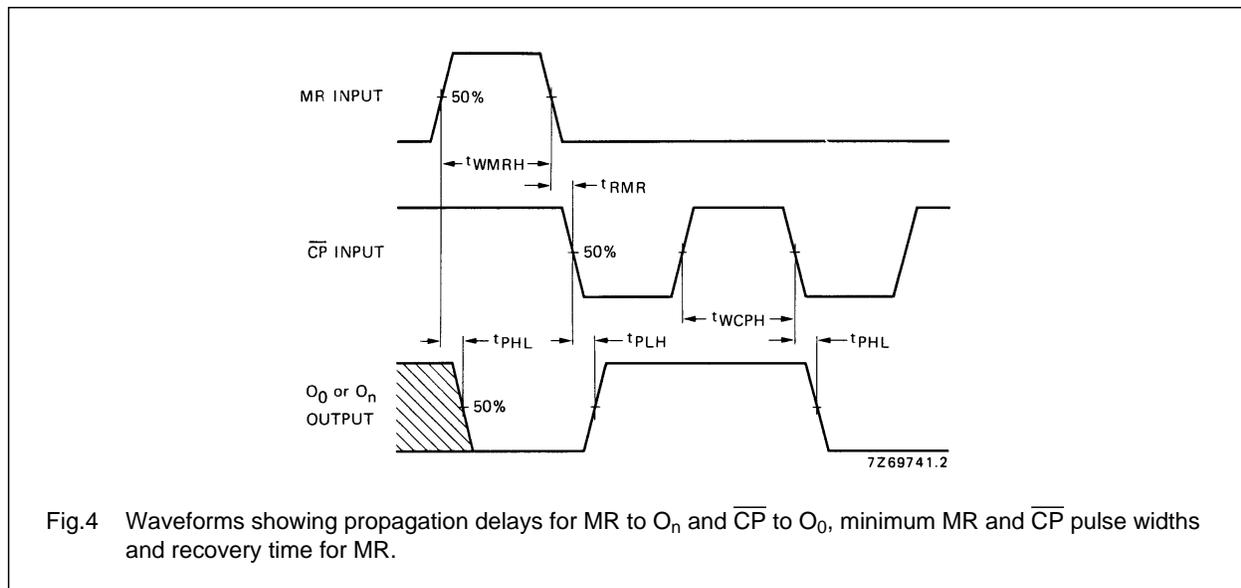
Fig.4 Waveforms showing propagation delays for MR to O<sub>n</sub> and CP to O<sub>0</sub>, minimum MR and CP pulse widths and recovery time for MR.
