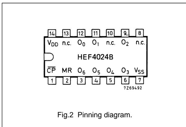
Fig.2 Pinning diagram.
