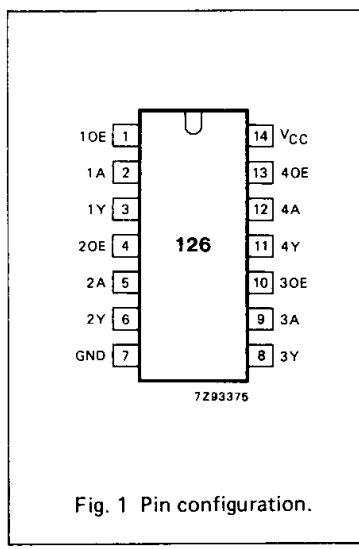
Fig. 1 Pin configuration.
