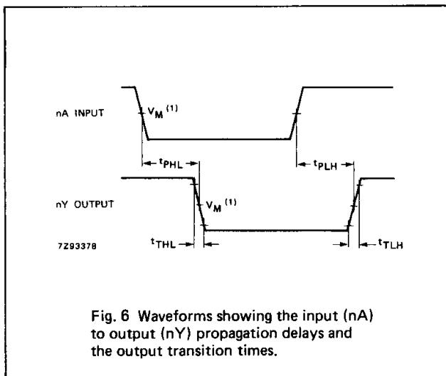
Fig. 6 Waveforms showing the input (nA) to output (nY) propagation delays and the output transition times.
