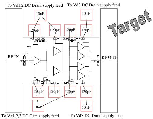
Note : Supply feed should be capacitively bypassed. 25µm diameter gold wire is to be prefered.
