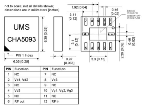
"Please note that PIN 1 is located in the lower left corner of the package (front-side view) for all SMD-type packages from United Monolithic Semiconductors. It is indicated by a triangle on the package lid. Starting with PIN 1 the other pads are numbered counter-clockwise (front-side view). ATTENTION: The dot on the backside of the package (i.e. side with metallic pads) is just for fabrication purposes and does NOT indicate the location of PIN
