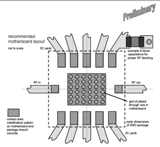
The RF ports comprise a DC blocking capacitor on chip level. The DC connections include a first level of DC decoupling capacitors (typically 120pF) in the package. However, all DC bias ports should be additionally connected to ground with 10nF capacitors at board level to prevent the MMIC from oscillations. These parts should be placed close to the SMD leadless package. If the same bias is required at different DC ports, the lines should only be connected behind these block capacitors.
