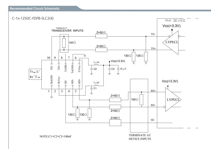
The split-loaded terminations for ECL signals need to be located at the input of devices receiving those ECL signals. The power supply filtering is required for good EMI performance. Use short tracks from the inductor L1/L2 to the module Rx Vcc. A GND plane under the module is required for good EMI and sensitivity performance.
