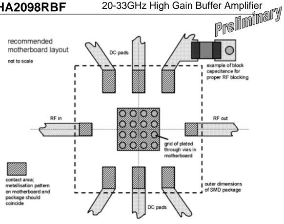
The RF ports comprise a DC blocking capacitor on chip level. The DC connections include a first level of DC decoupling capacitors (typically 120pF) in the package. However, all DC bias ports should be additionally connected to ground with 10nF capacitors at board level to prevent the MMIC from oscillations. These parts should be placed close to the SMD leadless package. If the same bias is required at different DC ports, the lines should only be connected behind these block capacitors.
