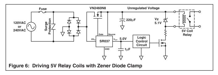
The circuit shown in Figure 6 uses the SR037 to supply a regulated 5.0V for the logic control circuitry. A 5.1V Zener diode is used in parallel with the 5.0V relay coil to ensure that the relay coil's maximum operating voltage is not exceeded. The Zener
