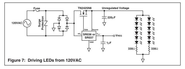
The circuit shown in Figure 7 uses the SR036 or SR037 to drive 12 high efficient red LEDs from a 120V AC line. The average LED current is approximately 20mA.
