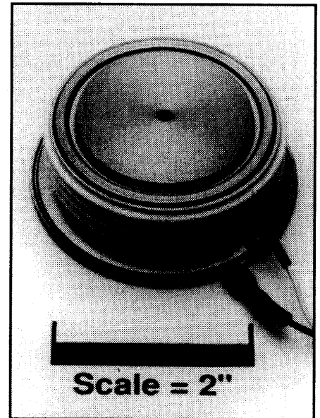
C451 Phase Control SCR 1500 Amperes Average, 2400 Volts
