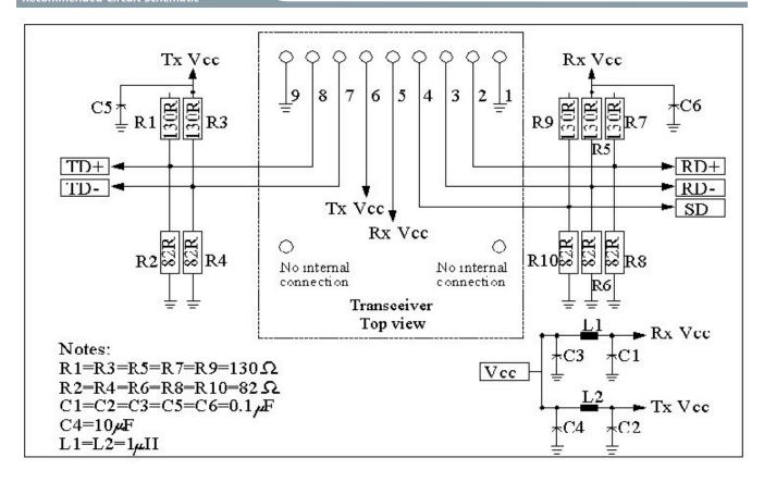
The split-loaded terminations for ECL signals need to be located at the input of devices receiving those ECL signals. The power supply filtering is required for good EMI performance. Use short tracks from the inductor L1/L2 to the module Rx Vcc. A GND plane under the module is required for good EMI and sensitivity performance.
