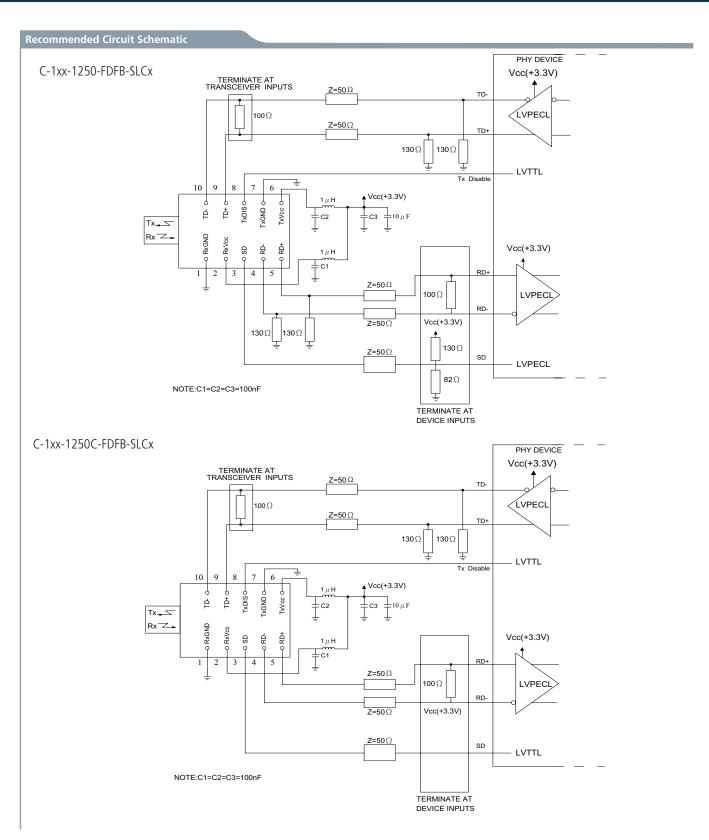
The split-loaded terminations for ECL signals need to be located at the input of devices receiving those ECL signals.
