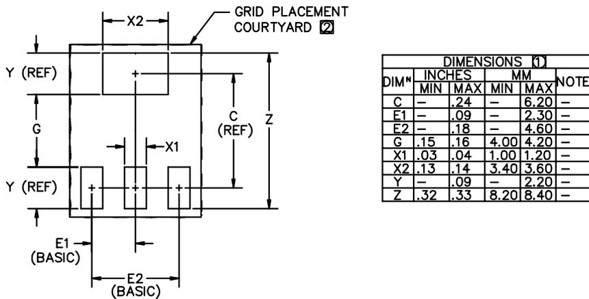
② GRID PLACEMENT COURTYARD IS 18 x 14 ELEMENTS (9 mm X 7mm) IN ACCORDANCE WITH THE INTERNATIONAL GRID DETAILED IN IEC PUBLICATION 97.
