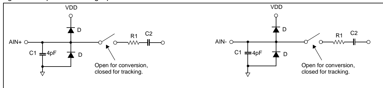
Figure 35. Equivalent Analog Input Circuit
