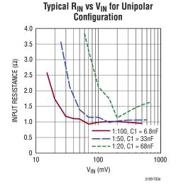
Using a 1:100 primary-secondary ratio yields start-up voltages as low as 30mV. Other factors that affect performance are the resistance of the transformer windings and the inductance of the windings. Higher DC resistance will result in lower efficiency and higher start-up voltages. The secondary winding inductance will determine the resonant frequency of the oscillator, according to the formula below.
