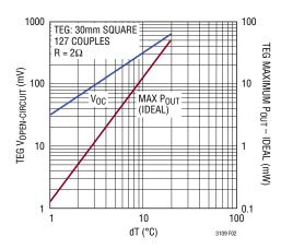
Figure 2. Typical Performance of a Peltier Cell Acting as a Power Generator (TEG)
