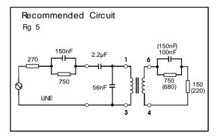
Figure 5 gives flat RX and TX responses against the reference impedance (typically around ±0.5dB 300Hz - 3.4kHz). Return loss is typically better than 20dB. The circuit values in parentheses give optimum flatness at a small sacrifice in return loss.
