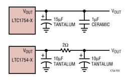
Figure 1. Output Ripple Reduction Techniques
