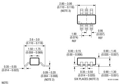
NUTE: 1. DIMENSIONS ARE IN MILLIMETERS 2. DIMENSIONS ARE INCLUSIVE OF PLATING 3. DIMENSIONS ARE EXCLUSIVE OF MOLD FLASH AND METAL BURR 4. MOLD FLASH SHALL NOT EXCEED 0.254mm 5. PACKAGE EIAJ REFERENCE IS SC-74A (EIAJ)
