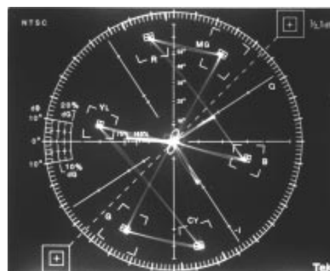
Vector Plot of Standard Color Burst
