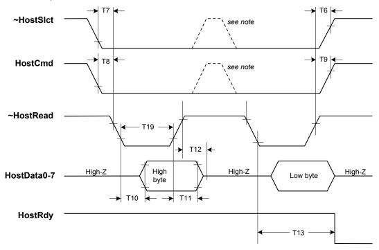
Note: If setup and hold times are met, ~HostSlct and HostCmd may be de-asserted at this point.
