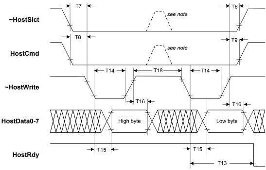
Note: If setup and hold times are met, ~HostSlct and HostCmd may be de-asserted at this
