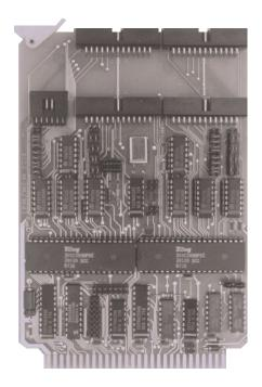
The LPM/MCM-7314 is a STD Bus and CMOS STD Bus compatible, four channel, RS-232-C input/output board, designed to be a multiprotocol asynchronous or synchronous serial communications board based upon the Z85C30 CMOS SCC. Each serial channel is
