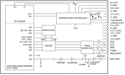
C7180 does not include the temperature controller and TE-cooler
