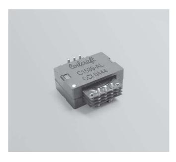
The C1539-AL was developed specifically for the National Semiconductor LM5032 dual interleaved current mode PWM controller. This planar transformer can be used in a dual forward converter or in both interleaved power stages of a high-current converter in applications up to 100 Watts.
