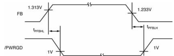
Figure 4. MIC2587/87R-2 FB to /PWRGD Timing
