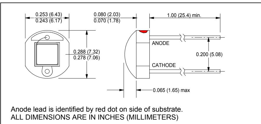
Anode lead is identified by red dot on side of substrate.
