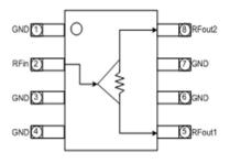
Pins 1,3,4,6 and 7 must be DC and RF grounded.
