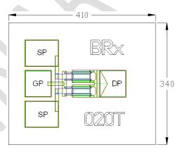
Chip dimensions: 410 X 340 microns Gate pad(GP): 75 X 75 microns Drain pad(DP): 75 X 75 microns Source pad(SP): 95 X 75 microns Chip thickness: 100 microns
