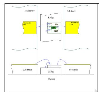
Using 1 mil. diameter, Au bonding wires.
