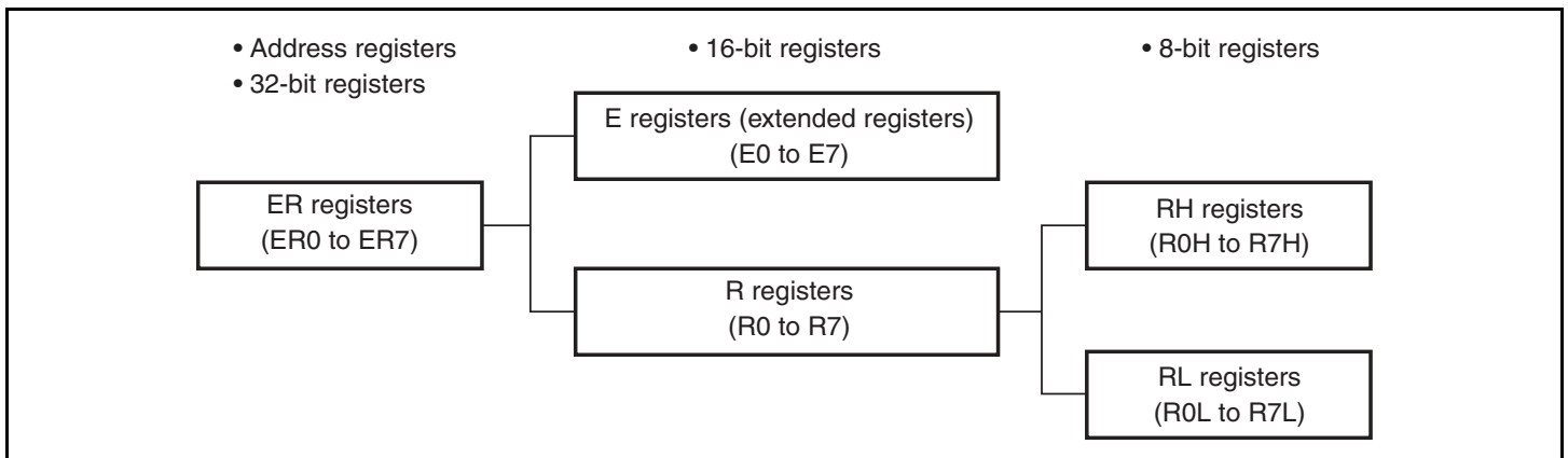
Figure 2.7 Usage of General Registers
