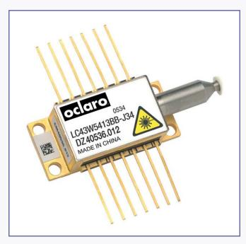
This laser module employs the Oclaro strained layer MQW Buried Heterostructure DFB laser chip, and is specifically for use in Wavelength Division Multiplexed (WDM) 4.25Gb/s Fibre Channel systems. The device is packaged in a hermetically sealed 14-pin butterfly package incorporating an isolator and monitor photodiode for control of the power of the laser over life and all operating conditions.
