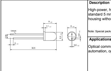
High-power, high-speed infrared LED in standard 5 mm package, wide beam angle, housing without standoff leads
