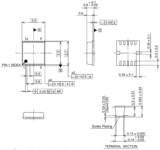
NOTE:1) The dimensions of the terminal section apply to the ranges of 0.1mm and 0.25mm from the end of a terminal.
