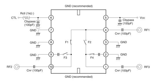
When using this IC, the following external parts should be used:
