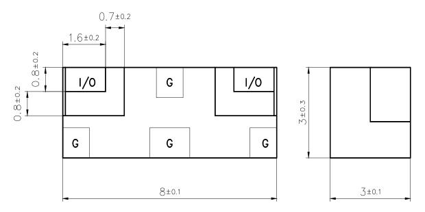
View from below onto the solder terminals and view from beside Marking: 'EPCOS logo '4007', on top of the filter
