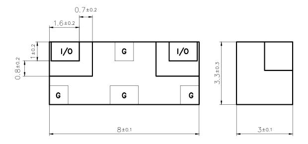
View from below onto the solder terminals and view from beside Marking: 'EPCOS logo '3707', on top of the filter
