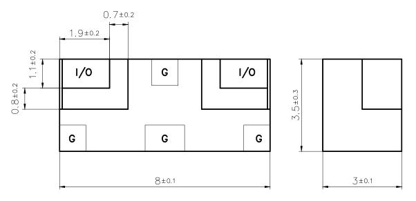
View from below onto the solder terminals and view from beside Marking: 'EPCOS logo '3557'', on top of the filter
